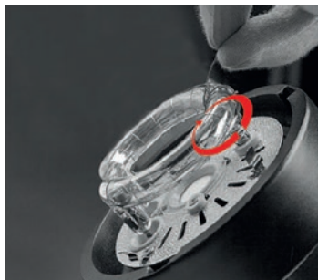
Fig. 1: Unwind the twisted ignition wire from the flash tube holder and carefully pull the flash tube out of the unit.
